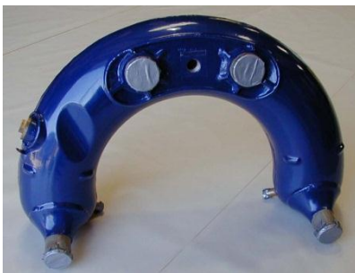
Figure 1. P-51 Header Tank
