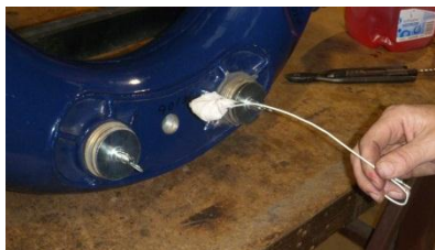
Figure 10. Inserting Swab into Header Inlet Ports
