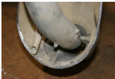
Figure 2d. Broken Welds at Outlet End of Scroll Tube
