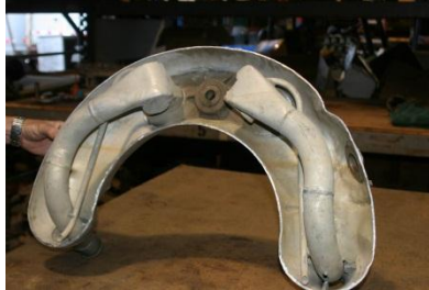
Figure 2a. Header Tank Internals
