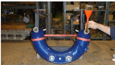
Figure 6. Inserting Fill Tube with Attached Funnel
