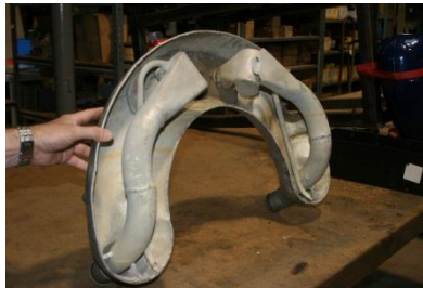
Figure 2b. Oblique View Showing Broken Scroll Chamber
