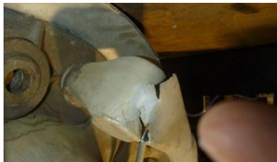
Figure 2c. Failed Header Tank Scroll Chamber
